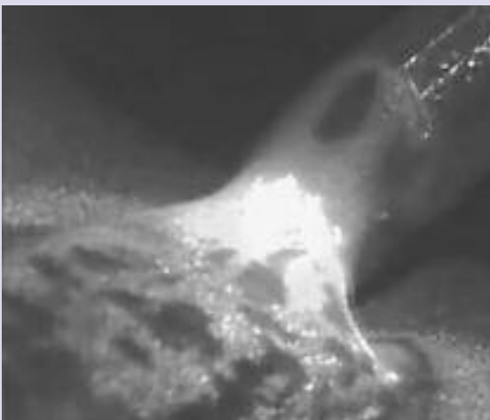
Individual frame of a high speed process analysis; the melting behavior, wetting and oxidation is clearly visible.
