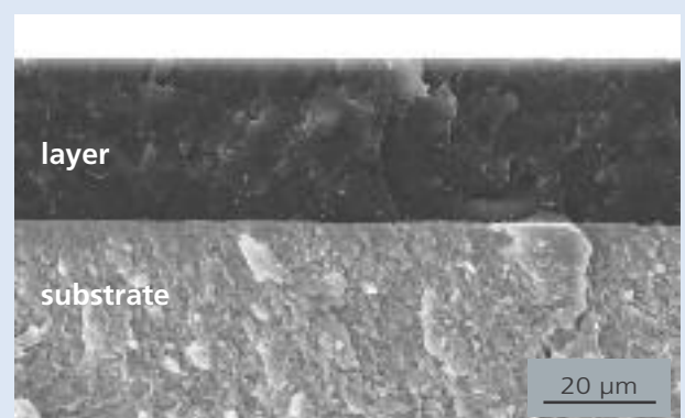
SEM cross-section image of a ta-C coating on a steel piston ring
